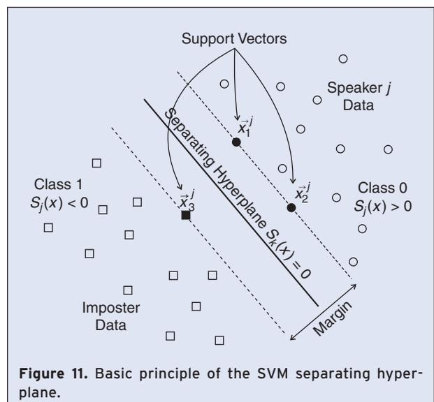
Figure 11. Basic principle of the SVM separating hyperplane.
