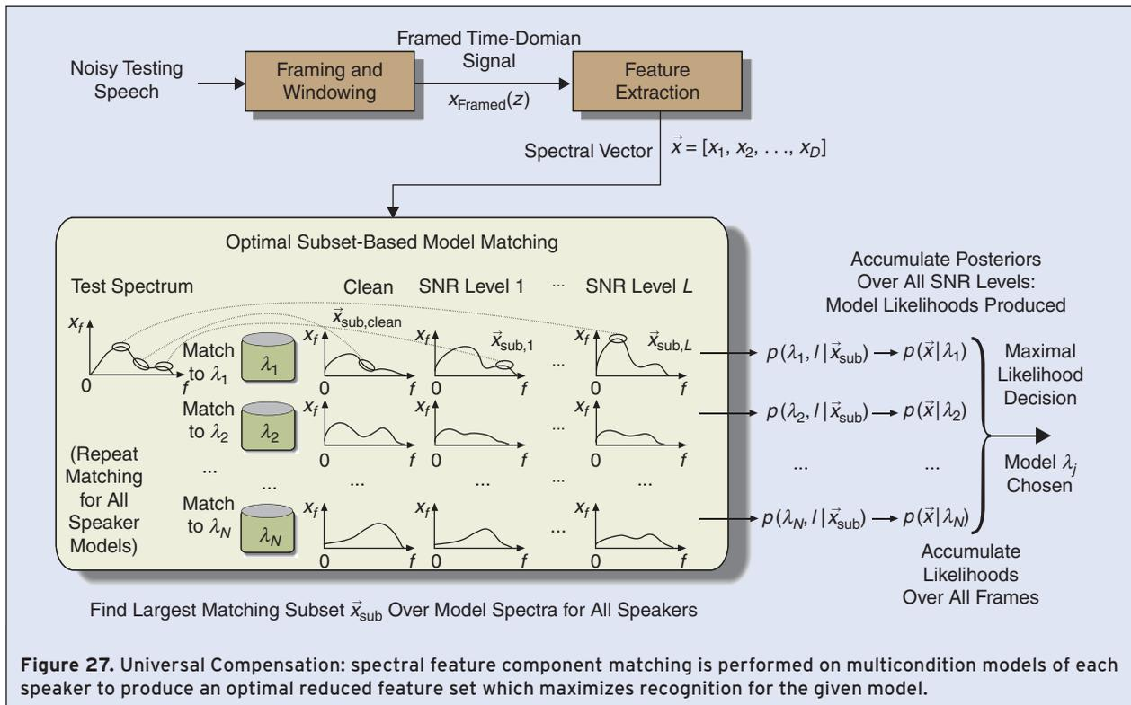
**Figure 27.** Universal Compensation: spectral feature component matching is performed on multicondition models of each speaker to produce an optimal reduced feature set which maximizes recognition for the given model.
