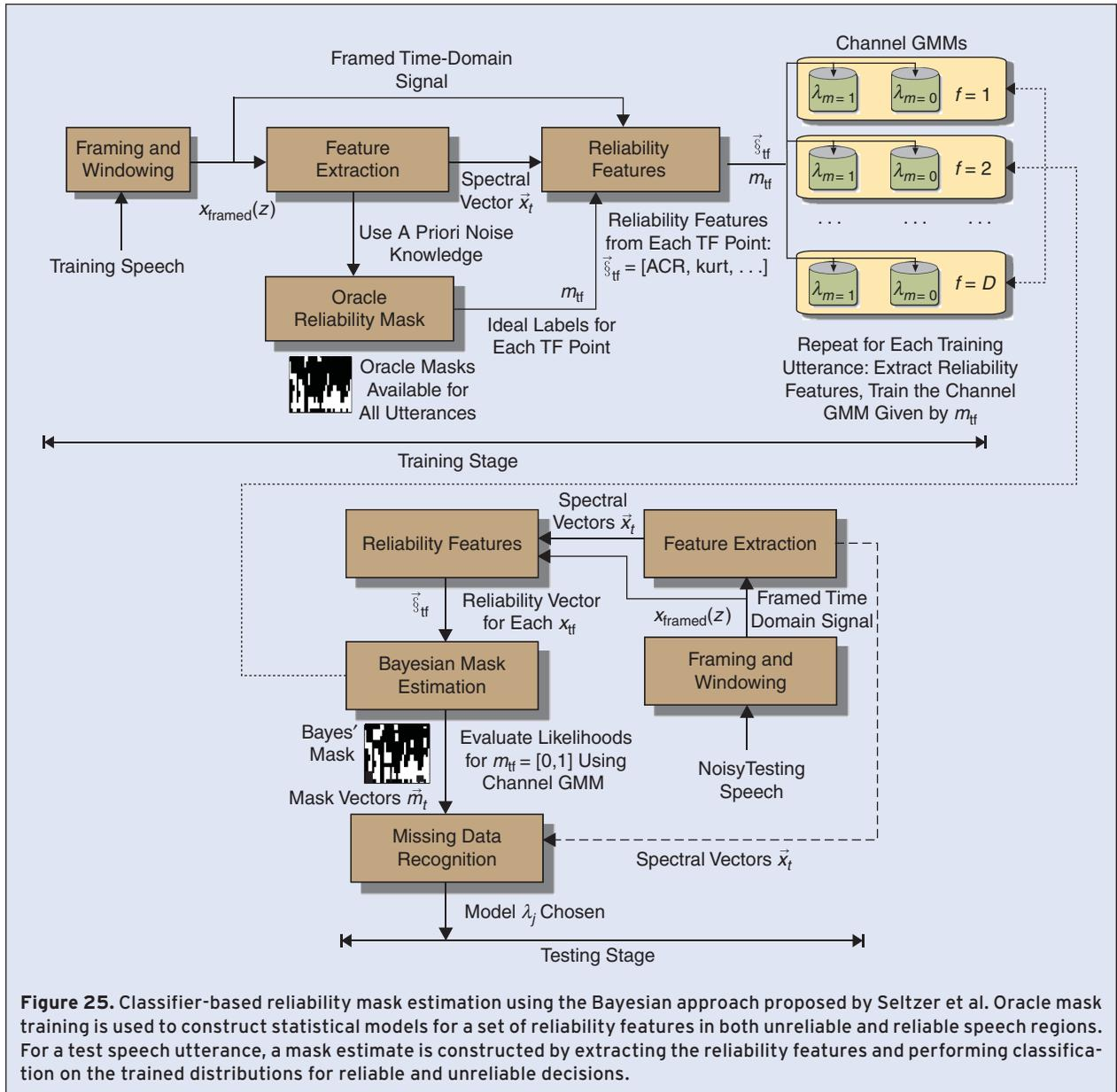
**Figure 25.** Classifier-based reliability mask estimation using the Bayesian approach proposed by Seltzer et al. Oracle mask training is used to construct statistical models for a set of reliability features in both unreliable and reliable speech regions. For a test speech utterance, a mask estimate is constructed by extracting the reliability features and performing classification on the trained distributions for reliable and unreliable decisions.
