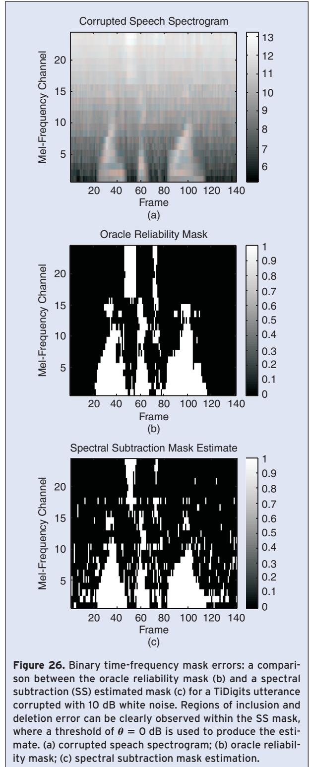
**Figure 26.** Binary time-frequency mask errors: a comparison between the oracle reliability mask (b) and a spectral subtraction (SS) estimated mask (c) for a TiDigits utterance corrupted with 10 dB white noise. Regions of inclusion and deletion error can be clearly observed within the SS mask, where a threshold of  $\theta = 0$  dB is used to produce the estimate. (a) corrupted speech spectrogram; (b) oracle reliability mask; (c) spectral subtraction mask estimation.
