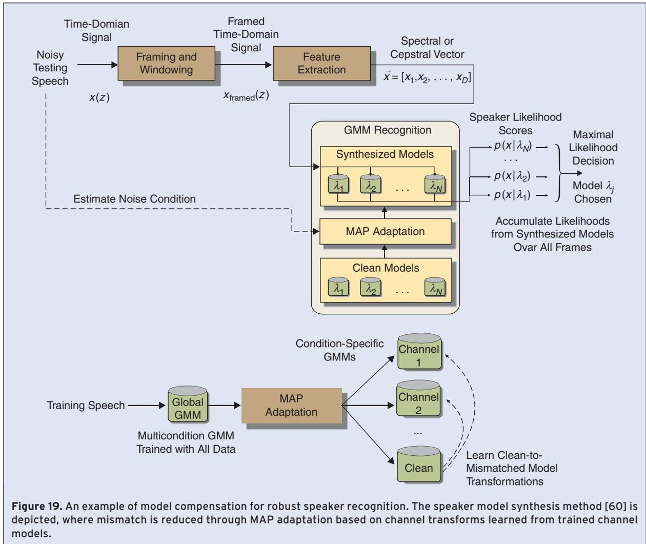
**Figure 19.** An example of model compensation for robust speaker recognition. The speaker model synthesis method [60] is depicted, where mismatch is reduced through MAP adaptation based on channel transforms learned from trained channel models.
