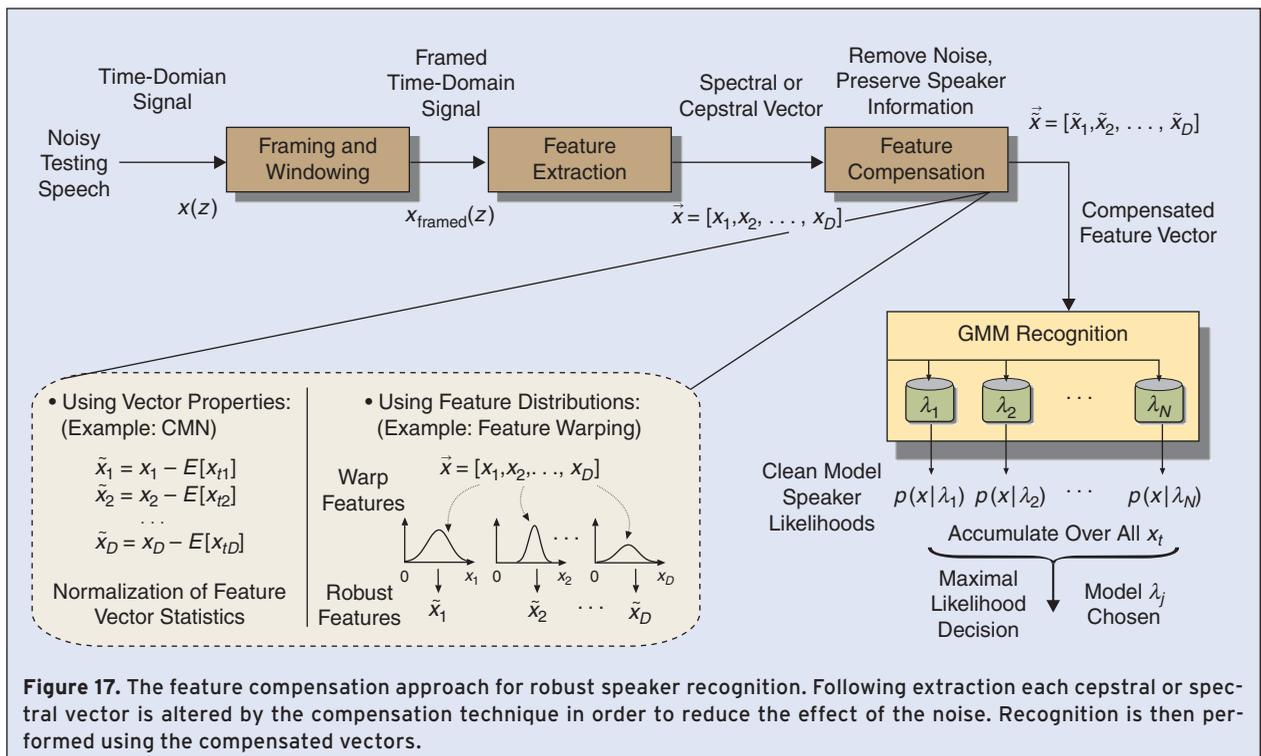
**Figure 17.** The feature compensation approach for robust speaker recognition. Following extraction each cepstral or spectral vector is altered by the compensation technique in order to reduce the effect of the noise. Recognition is then performed using the compensated vectors.
