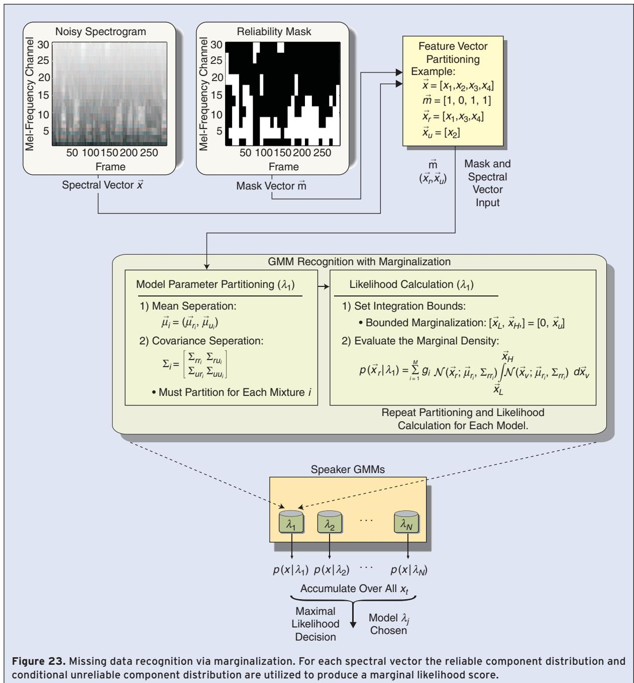
**Figure 23.** Missing data recognition via marginalization. For each spectral vector the reliable component distribution and conditional unreliable component distribution are utilized to produce a marginal likelihood score.
