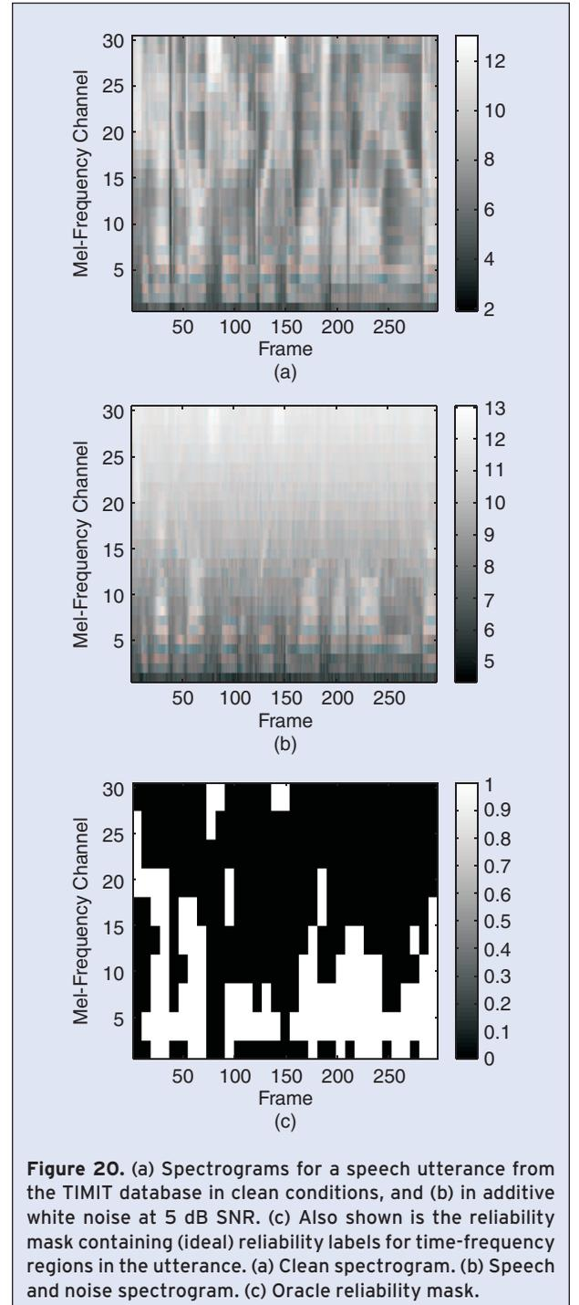
**Figure 20.** (a) Spectrograms for a speech utterance from the TIMIT database in clean conditions, and (b) in additive white noise at 5 dB SNR. (c) Also shown is the reliability mask containing (ideal) reliability labels for time-frequency regions in the utterance. (a) Clean spectrogram. (b) Speech and noise spectrogram. (c) Oracle reliability mask.
