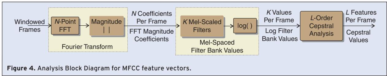
Figure 4. Analysis Block Diagram for MFCC feature vectors.
