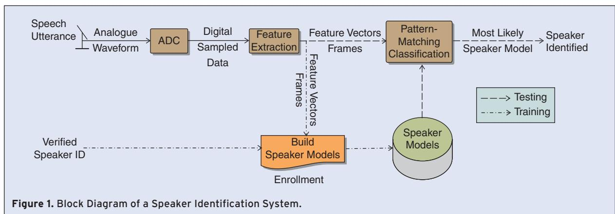
**Figure 1.** Block Diagram of a Speaker Identification System.
