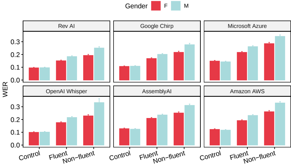
Fig. 10. On a total sample of 1,843 control, 2,393 fluent aphasia, and 1,392 non-fluent aphasia audio files, we find that WER is consistently worse for non-fluent aphasia speakers compared to fluent aphasia speakers. A more granular analysis of WER by gender reveals that WER is consistently worse for male (M) aphasia speakers compared to female (F) aphasia speakers across all ASR services, and the difference is compounded for speakers with more severe aphasia (i.e., the gender performance gap is more severe for non-fluent aphasia speakers than for fluent aphasia speakers). There were no non-binary speakers in our data sample.
